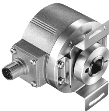
The SinCos feedback system is a combination of incremental sensor and absolute sensor. The absolute value is initially only defined when the device is switched on and transmitted to an external counter, which then continues counting incrementally from this absolute value with the analogue Sinus/Cosinus interface.
