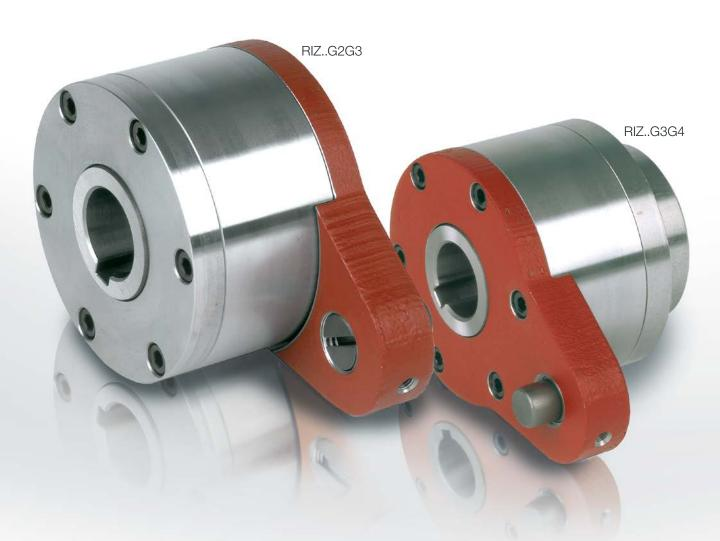
Types RIZ..G2G3/G3G4 are centrifugal lift off sprag type freewheels with the inner race rotating. Only the inner race is designed for freewheeling.
