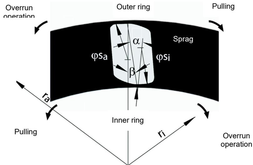
Fig. 2 Pulling/Overrun operation
