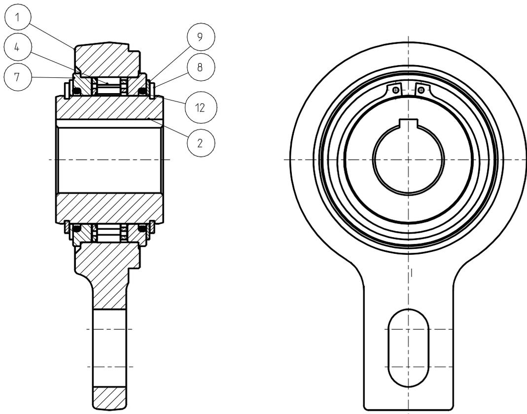
Fig. 1 Structure of one-way clutch RSBW
