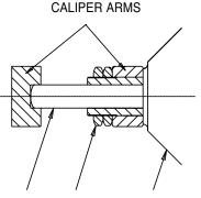
PUSHROD LOCKNUTS THRUSTER
