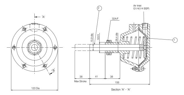
This range of pneumatically operated brakes uses dry and filtered compressed air at pressures up ot 7 bar. Pneumatic brakes require a control valve which may be operated either manually, or by pneumatic or electrical signal.
