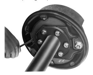
Figure 4 - Brake Adjustment
