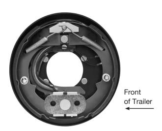
Figure 2 - Mounting Position
