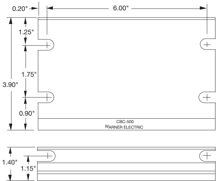
This control may be mounted on its base (two mounting slots) or on its back (four mounting slots).
