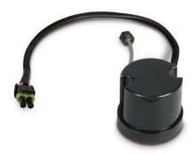
The P2.0 Position Control is a microprocessor position feedback control providing a 0-10 volt DC output indicating actuator travel. The control uses two inductive pulse count sensors and a counting wheel to accurately determine actuator position. A third sensor at the full retract position provides a zero or home position indication.
